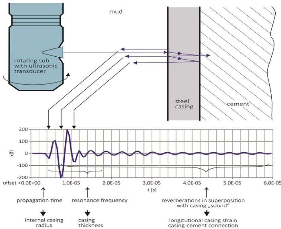
Fig. 1 Schematic of ultrasonic wave propagation from transducer to borehole casing, interaction with the casing (reverberations), backscattering of the signals to the transducer. From the received full waveform information on internal radii, thickness, casing-cement connection and longitudinal casing strain are deduced [1]
