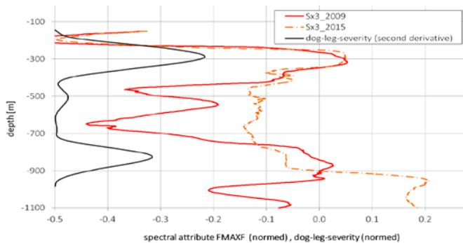
Fig. 5 Spectral attributes FMAXF of borehole Sx3. The log from 2009 (full red line) does follow the dog-leg severity (black line, see Fig. 6). The log from 2015 fits with the older log from the surface to a depth of 450 m, at higher depth the values increase significantly (dashed line)
