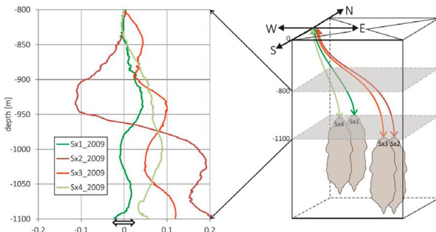
Fig. 7 Comparison of spectral attribute FR(FMAXF) vs. depth in the interval 800–1100 m for four borehole casings. At a depth of 1100 m there is a clear separation of values ( $Sx1 < 0$ ,  $Sx2, Sx3, Sx4 > 0$ ) detectable. Spectral attributes greater than zero are understood as lengthening of the borehole casing. Their drilling paths following NW–SE direction which are overlaid by local stress in the same direction.
