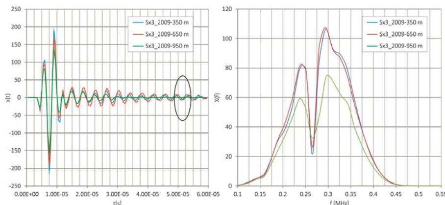
**Fig. 2** Signal processing of cavern Sx3 for three single traces in different depths: amplitude vs. time (left) and spectral amplitude vs. frequency. In the tail part of the time-signal (marked) there is a phase shift detectable. In the cone-like spec-tra of these traces both the resonance frequency of 0,270 MHz and a frequency shift especially on the lower-frequency flange are detectable
