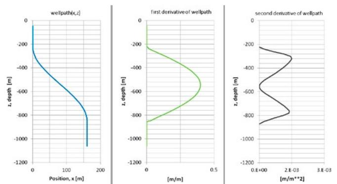
Fig. 6 Simplified example of the first and second derivative of the borehole path (x,z) of a S-shaped borehole
