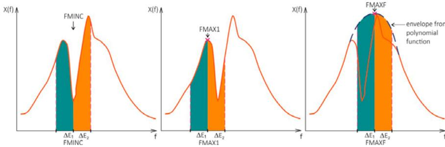
Fig. 4 Definition of criteria for spectral attribute characterization based on fixed frequencies: FMINC, main resonance frequency (left); FMAX1, first local peak below the main resonance frequency (middle); FMAXF, frequency of the peak envelope (right). The quotient of the energy containing the lower and upper frequency bands is called Differential Frequency Ratio (DFR)
