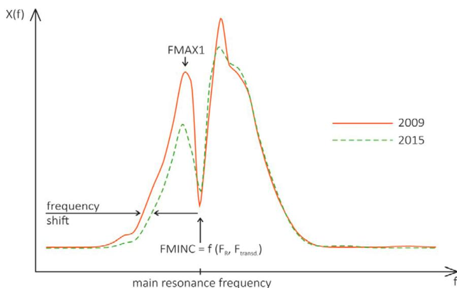
**Fig. 3** Frequency spectra from cavern Sx3 logged in the same depth at different times. The frequencies for FMAX1 and FMINC are invariable. At lower frequencies there is a frequency shift between 2009 and 2015 towards higher frequencies detectable
