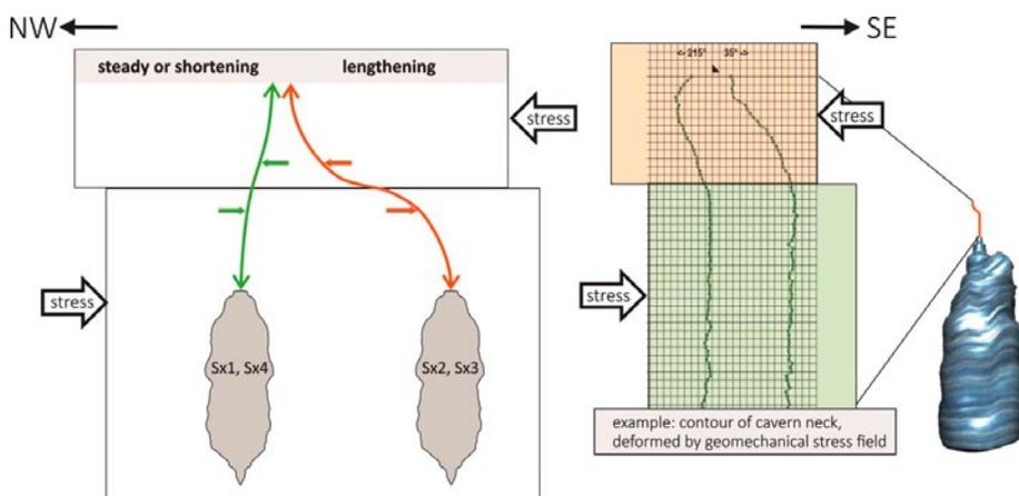
Fig. 8 Geological situation: local stress field from NW to SE causes lengthening of SE-deviated borehole casings ( $Sx2, Sx3$ ). Boreholes deviated in N or NE direction ( $Sx1, Sx4$ ) are less influenced by local stress field resulting in shortening or constant casing length. On the right the result of measured cavern neck deformation of a neighbored cavern in the same field is shown. Originally the cavern neck was a vertical borehole section of diameter 19"
